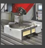
Integrated work of divisor with the system supplies 5 axis ability to the system
